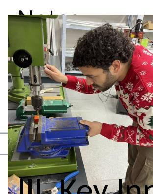
Most structural parts were FDM-printed; load-bearing interfaces were reinforced with steel pins and standard fasteners. Critical holes were drilled or reamed after printing to improve alignment and reduce friction. The prototype was assembled in modules to support fast repair and parameter tuning.
