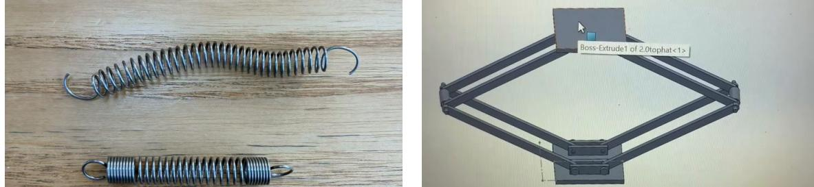
The robot employs a two-leg four-bar linkage that amplifies stored spring energy into a fast extension at the foot. A geared motor charges the springs through a compact latch; the latch is released to initiate a jump. The design prioritizes low mass, modularity, and rapid iteration with 3D-printed components.
